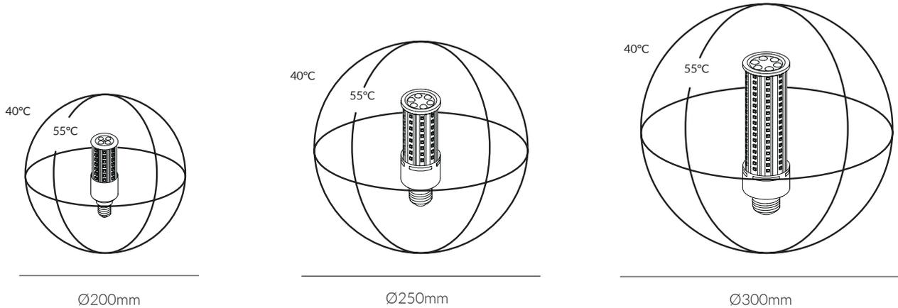
Approximately spherical, thin (1-5mm) glass or plastic diffusers
